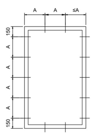
The illustration above is a general guideline for installation. If a different distance between fixing points has been calculated for the relevant project, the calculated distance shall be applicable.
