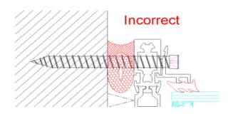
2. Next step is the Installation of the cap profile. Use a rubber or plastic hammer. The correctness of the installation of the cover can be checked easily. If cap is installed correctly, then the face of the cap must be lower than the face of the frame or transom.
