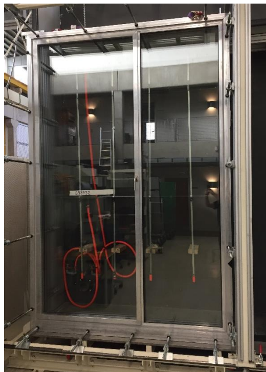
Door height window during testing
